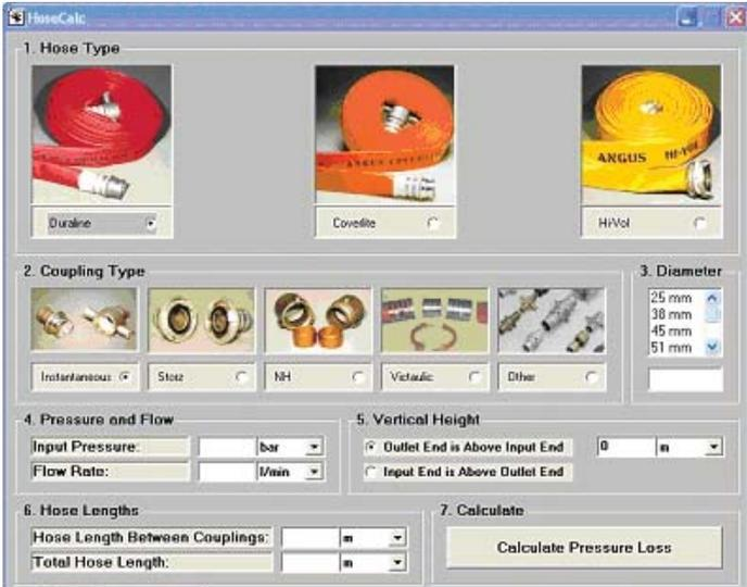
Pressure is also needed to overcome the friction in every bend, coupling and dividing breeching in the discharge hose. If too many bends, couplings and other obstacles are included the pressure losses may be too great for the pump to overcome and little or no water will flow.
